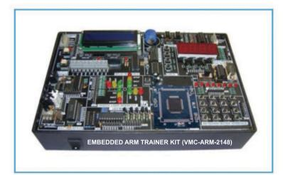
VMC-ARM-2148, the Embedded Arm Trainer has been designed by using Philips LPC214X Microcontroller. This controller provides in-system as well as in circuit programming so that one may be able to write program and download directly in the controller through serial port without removing it from the system.
