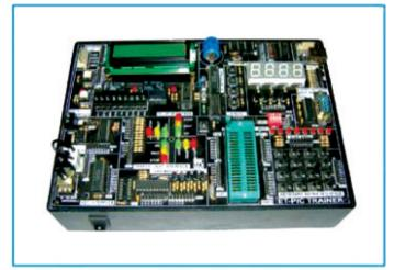
VMC-ET-PIC87X, the low cost Embedded Trainer has been designed by using Microchip PIC16F877 Microcontroller. This controller provides in-system as well as in circuit programming so that one may be able to write program and download directly in the controller through serial port without removing it from the system.
